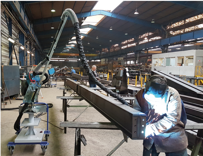
Swing arm EQU21 on trolley EQU0R
