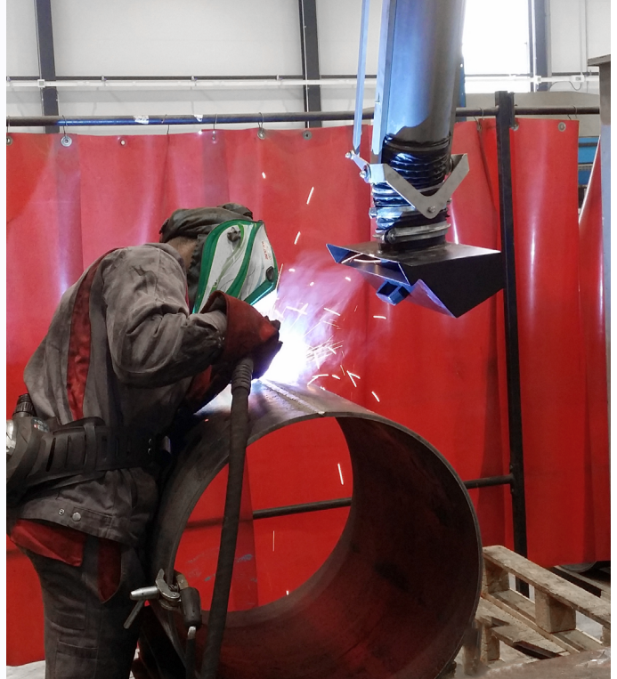
Extraction arm ARMOWELD with slit nozzle REVOLFLOW
