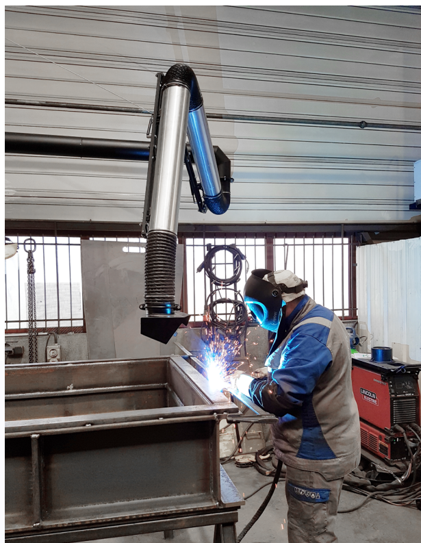
Extraction arm ARMOWELD with laminar flow nozzle REVOLFLOW
